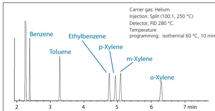
Figure 8. Chromatogram showing separation of a BTEX mixture using a SolGel-WAX™ column (30 m x 0.25 mm ID x 0.25 μm film thickness).
