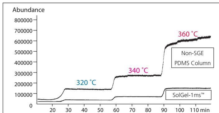
Figure 4. Bleed chromatograms generated from a commercially available poly(dimethylsiloxane) (PDMS) column (top) and a SolGel-1ms™ column (bottom) using a mass selective detector. Both columns were 30 m x 0.25 mm ID x 0.25 µm film thickness.
