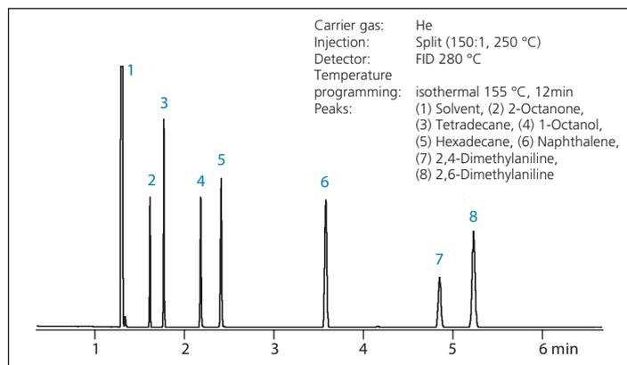
Figure 5b. SolGel-WAX™ column (30 m x 0.25 mm ID x 0.25 µm film thickness) after heating at 250 °C for 1 hour with the carrier gas turned off.
