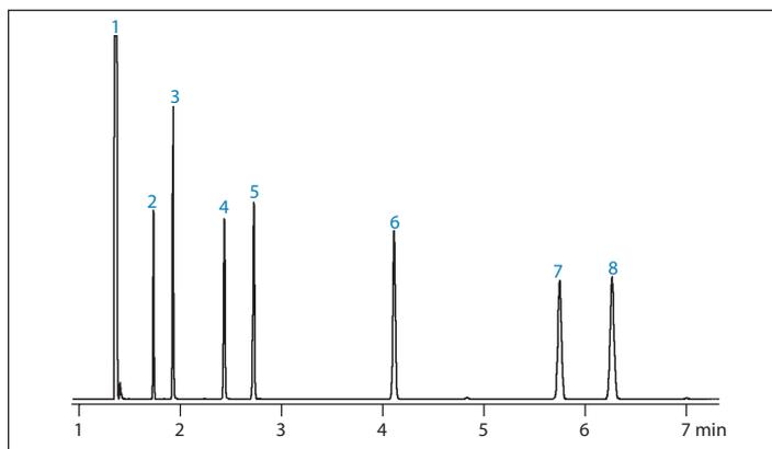
Figure 5a. Separation of a selection of compounds using a SolGel-WAX™ column (30 m x 0.25 mm ID x 0.25 µm film thickness), before heating at 250 °C for 1 hour with the carrier gas turned off.
