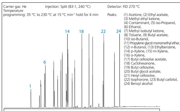
Figure 7. SolGel-WAX™ column (30 m x 0.25 mm ID x 0.25 μm film thickness) after heating at 250 °C for 1 hour with the carrier gas turned off.
