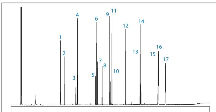
Figure 3a. The chromatogram shows separation of a selection of compounds from the US EPA 8270 semi-volatiles method using a SolGel-1ms™ column (30 m x 0.25 mm ID x 0.25 µm film thickness).
