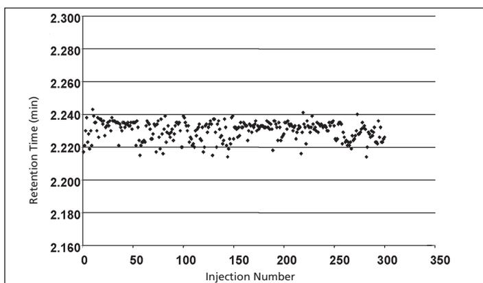
Figure 6. Graph showing the retention times of acetone in water over 300 injections using a SolGel-WAX™ column (30 m x 0.25 mm ID x 0.25 μm film thickness).
