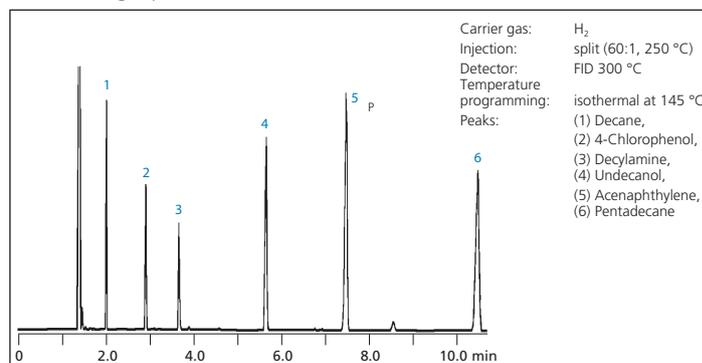
Figure 2. Standard test mix run on a SolGel-1ms™ column (30 m x 0.25 mm ID x 0.25 µm film thickness).
