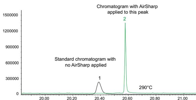
Figure 2. Overlaid chromatogram of a high boiling point compound that has not been subjected to AirSharp (1) and the same peak after AirSharp was applied (2).
