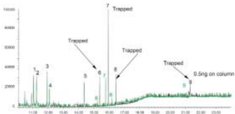
**Figure 5.** Overlaid chromatograms of the standard chromatogram of the horse racing mixture (in green) and the AirSharp focused chromatogram (in black) at 0.5 ng on column. Note the improved signal to noise ratio of the peaks subjected to AirSharp focusing and the distinguishing the peaks of interest from that of the baseline noise.
