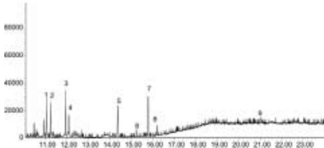
**Figure 4.** Chromatogram of the horse racing mixture at 0.5ng on column. Notice the low response of Dilantin (6), Nordiazepam (8) and Diphenoxylate (9).
