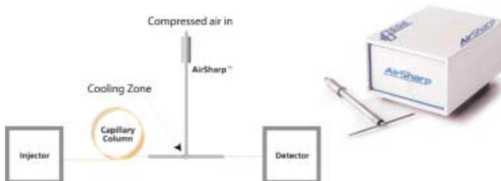
**Figure 1.** Picture of the cooling apparatus of the AirSharp and note its positioning near the end of the capillary column and before the detector. The capillary column passes through the tubing at the bottom and the compressed air is blown in from the top cooling the outside of the capillary column. Also a picture of the AirSharp control module.
