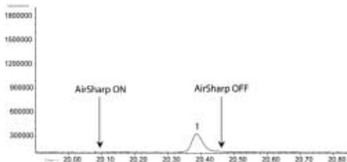
Figure 3. Chromatogram of when to turn the AirSharp on and off with respect to the elution of the targeted peak.
