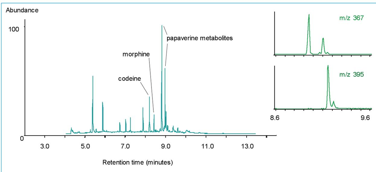
**Figure 1b:** The analysis of enzyme hydrolyzed horse urine by GCMS following micro-SPE extraction and micro-derivatization (peracetylation) of the recovered basic fraction. (Inset m/z 367 corresponds to O-desmethylpapaverine metabolites and m/z 395 is the O,O'-didesmethylmetabolites)
