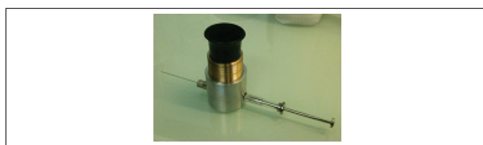
Figure 1. Magnifying tool developed to improve the accuracy, precision and consistency of syringe use.
